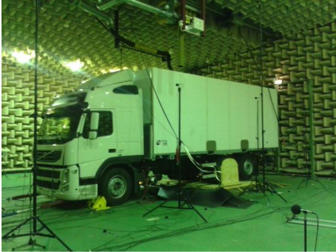
Figure 3, Project truck in the Semi-Eco free room at Volvo Noise and Vibration Laboratory.
