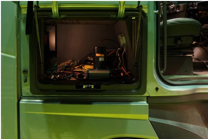
Figure 6-4 The physical installation of the prototype equipment in one of the demonstrator trucks.
