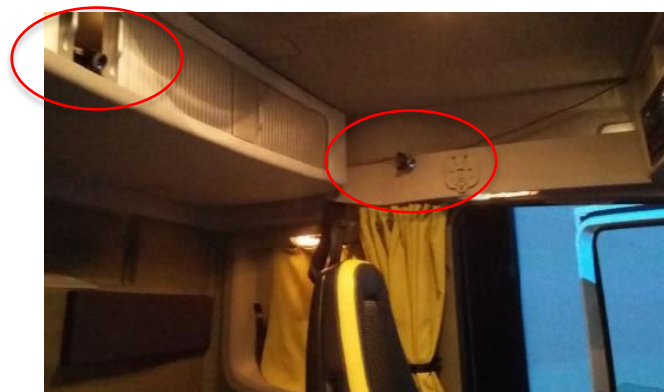
Figure 6-2 Cameras mounted in the cab to monitor the driver
