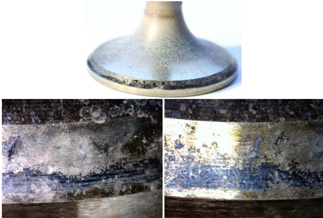
Figure 6. Examples of valves tested in the rig, using a flow of oil mist that has resulted in the formation of tribofilms. Top: overview. Left: valve run 100 000 cycles (i.e. as many cycles as in Fig. 4d) Right: valve run 500 000 cycles. Extremely low wear compared to the valves run in air.
