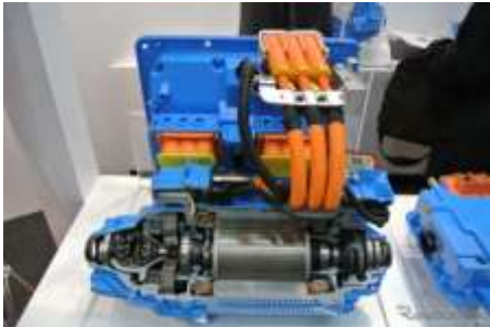
FIGURE 2, DRIVE PACK WITH ELECTRIC MACHINE, CONVERTER AND CLUTCH
