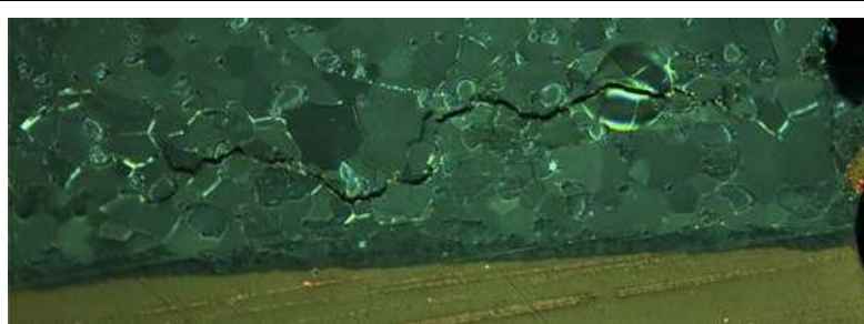
Figure 2. Example of crack propagation after temperature cycling of BGA component.
