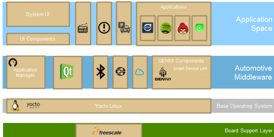
Figure 5: PLINTA reference system overview.
