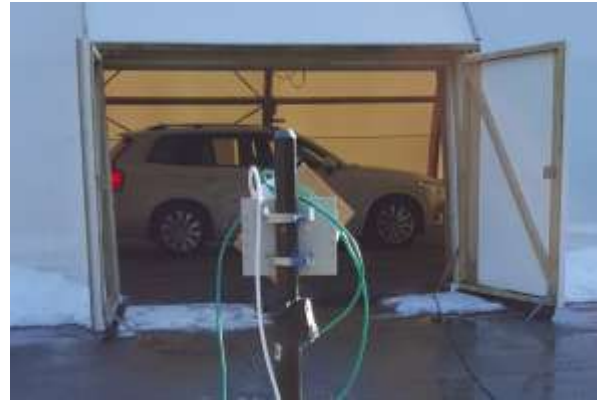
Figure 6 TX/RX experiment for 24/60 GHz Band
