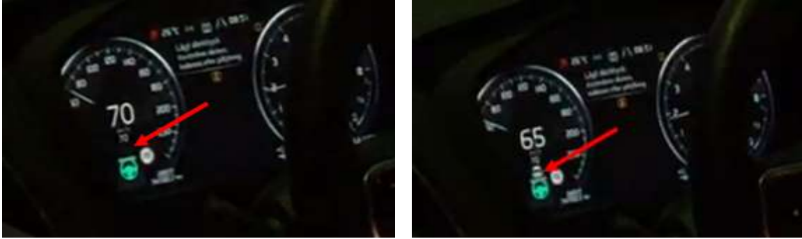
Figure 6: Driver information display, before and after the radar target has appeared in front of the car.
