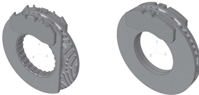
Figure 1. Left: The assembly of the disc-pad system with a disc shown sectioned. Right: The assembly of the disc-pad system after removing the geometry not considered important for the simulation
