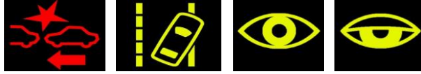
Picture 4. Warning symbols for collision, lane departure, distraction and sleepiness, displayed on the screen mounted in the dash board
