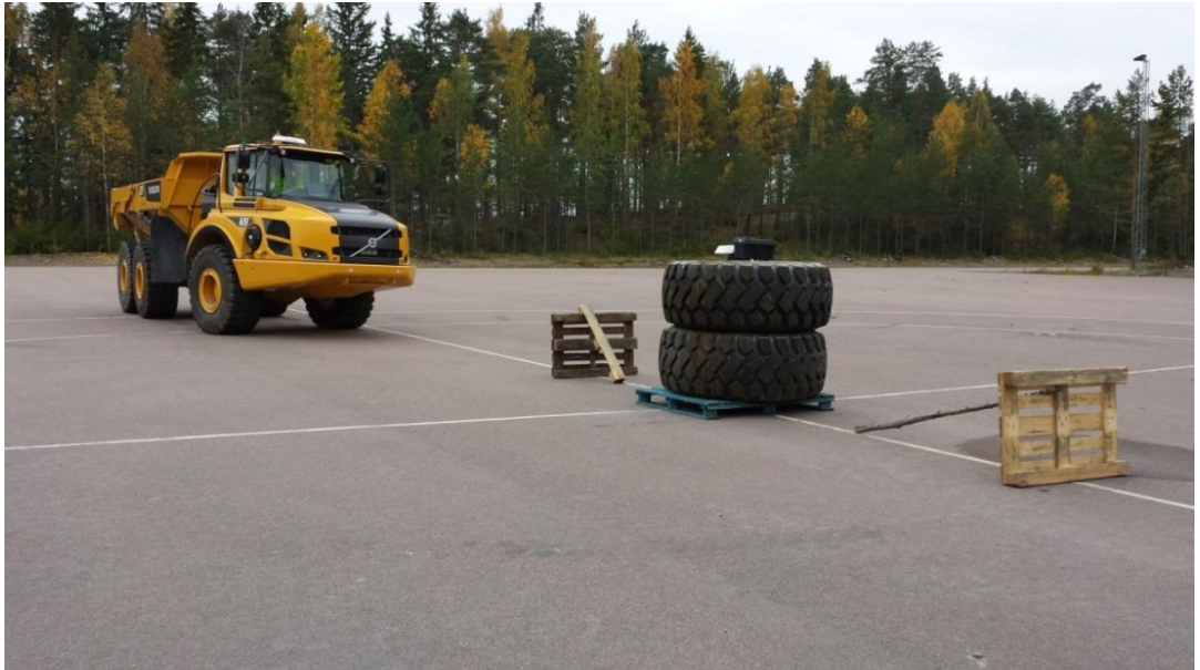
Figure 2: Testing of emergency brake on A25 Hauler in Eskilstuna. The positioning units can be seen on top of the machine and on the pile of tires. To avoid damages to the equipment in case of missed interventions, some safety margins were added around the object antenna as indicated by the pallets.
