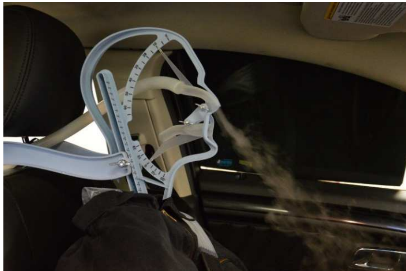
Fig 6. Vehicle compartment flow experiments were conducted using a model of a breathing human being.
