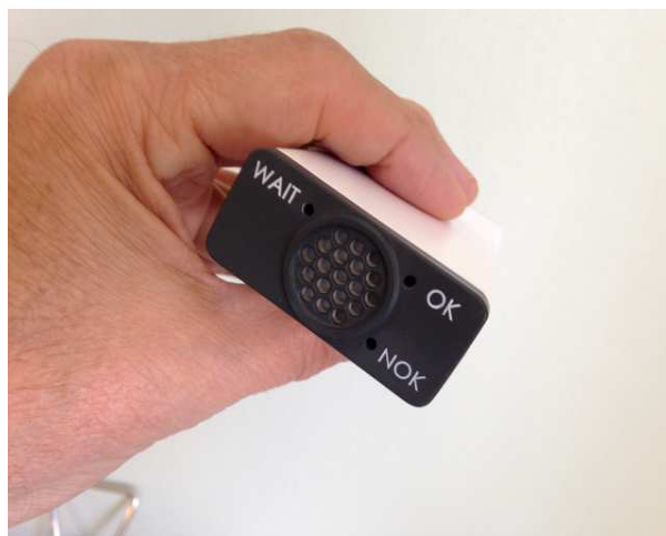
Fig 5. Example of user interface based LEDs
