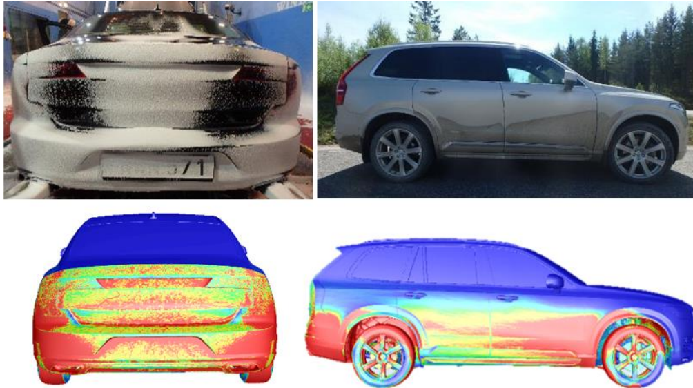
Figure 12. Wind tunnel tests for snow and gravel tests compared to results from CFD
