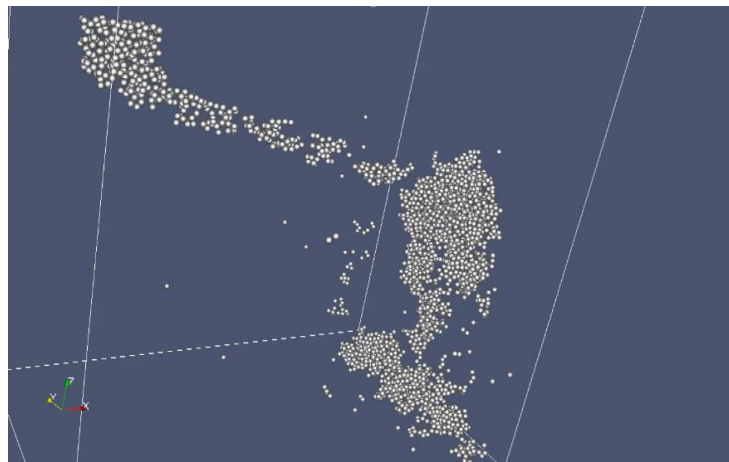
Figure 7. DEM particle impingement model to evaluate adhesion conditions
