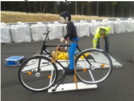
Figure 6. Vehicle platform ABD GST with bicycle target mounted with an offset.
