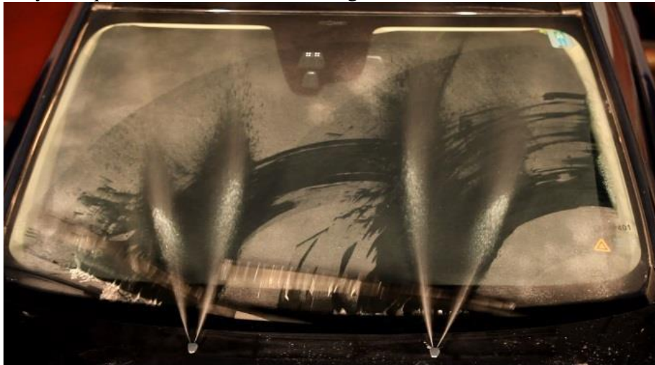
Figure 2 Wind screen and sensor cluster cleaning at high wind speeds. Full scale wind tunnel tests – Volvo Cars.
