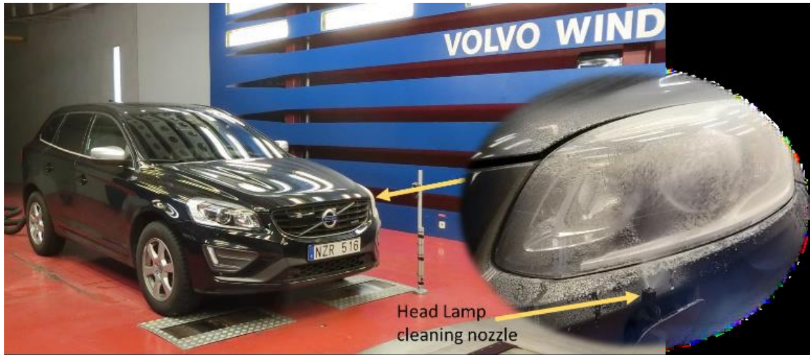
Figure 4 Full scale Head Lamp Cleaning test for a Volvo XC60, courtesy of Volvo Cars
