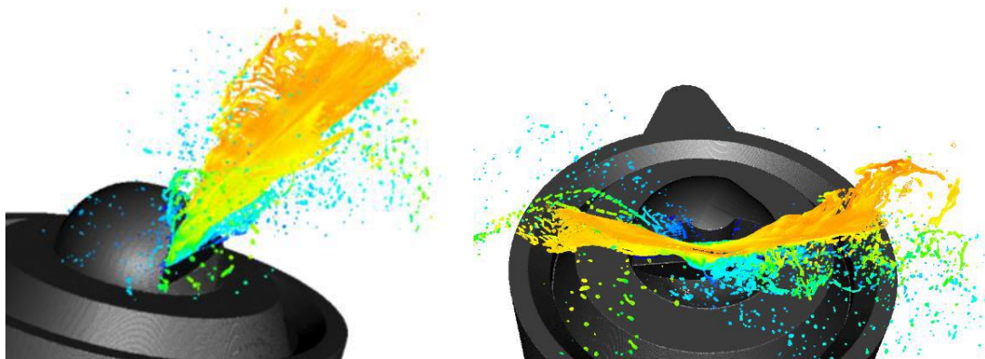
Figure 3 Side and top view of a conventional nozzle discharging cleaning liquid
